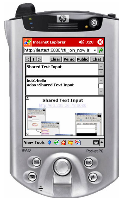
Fig. 1. The shared text input system accessed from a PDA. Users can quickly type in notes by re-using words from the slide image (bottom) or from the notes taken by their friends (middle). Users simply tap the desired word to paste it into their notes.
