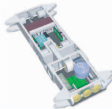
Fig. 12. Another innovation in Whegs TM IV is a clear acrylic front panel. This makes it possible to mount infrared sensors or a video camera internally in an area directly adjacent to the main electronics compartment. The rounded shape of the front Panel will have good hydrodynamic characteristics and will also allow it to push up and over irregularly shaped obstacles
