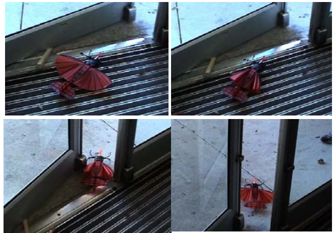
Fig. 6: When (a) MMALV is confronted with a narrow passage, it (b) retracts its wings, (c) negotiates the passage, and (d) redeploy its wings.
