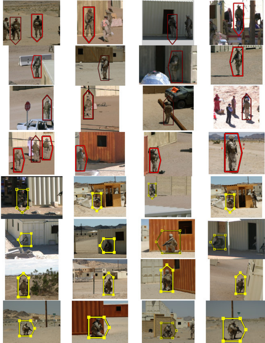
Figure 7. Examples of detections: Each row of images shows the detection of one specific class. The first four classes are ordered from top to bottom as following: standing 0, 90, 180, 270 degrees torso. The last four classes are, from top to bottom: kneeling 0, 90, 180, 270 degrees torso. The color of the bounding box is red for standing and yellow for kneeling. The orientation is expressed by the direction of the arrow within the bounding box. The boldness of the bounding box is proportional to the score of the detection.
