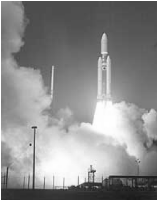
Figure 2: A Titan IVB missile launches a satellite from Cape Canaveral. This expendable launch vehicle can boost up to 47,800 pounds into low-Earth orbit or more than 12,700 pounds into geosynchronous orbit 22,300 miles above Earth. The payload joins a constellation of similar satellites that Space Command uses to provide early warning of missile launches worldwide (US Air Force 2001). The launcher and the satellite are components of separate space systems, but the satellite requires the launcher.
