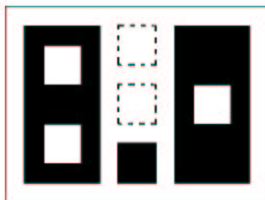
Figure 1.9. An example vehicle “hat” (number 1 shown). The large “blobs” are used to determine vehicle location and orientation and the smaller blobs determine the vehicle’s identity.
