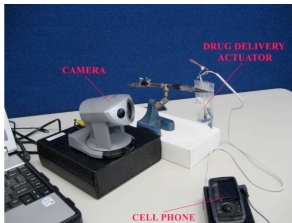
Figure 3. Network-controlled drug actuator setup
