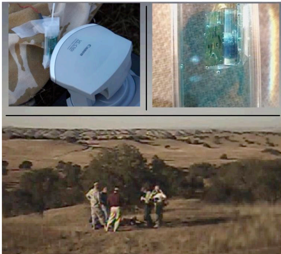
Figure 4. TOC Video Wall view of the casualty simulation mannequin and first release of liquid drug into vial (up-right corner of picture) upon voice activation from the medic's Blackberry handheld.
