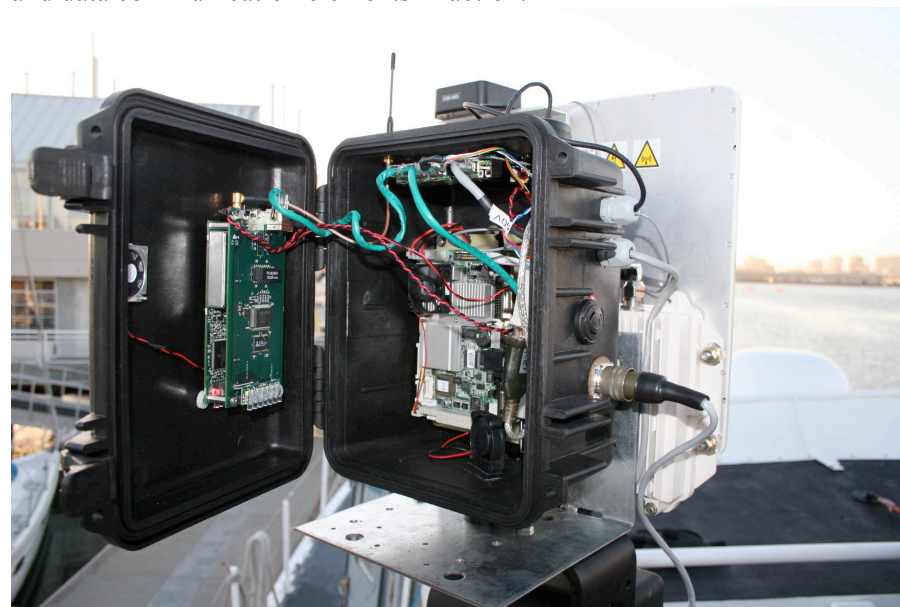
Figure 15. Basic components of SAOFDM node deployed to the Boarding Vessel.
