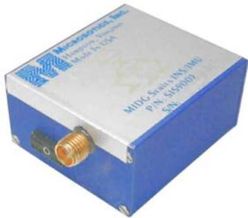
**Fig. 11** The Microbotics IMU.
