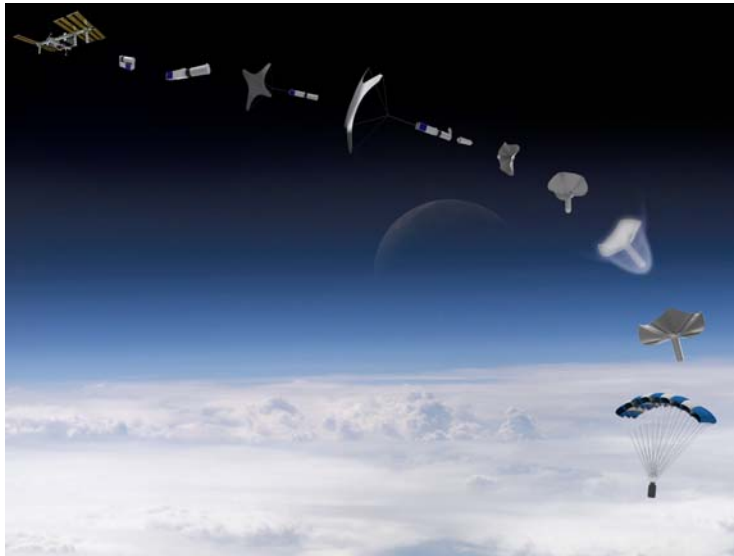
Fig 1. Pictorial overview of SPQR on-demand payload delivery system concept, from ISS deployment to atmospheric descent.
