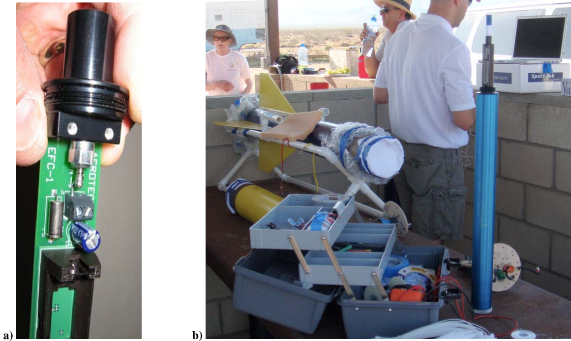
Figure 6. G-Triggered igniters (a) and loaded booster motor and igniter (b).
