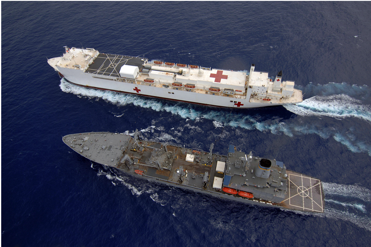
Figure 4. USNS Mercy (T-AH-19) and USNS Pecos (T-AO 197) demonstrate various configurations for helicopter landing deck placement. Official U.S. Navy photograph by Chief Photographer's Mate E. G. Martens.
