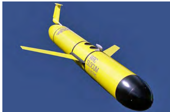
Figure 3.1: The Slocum Glider manufactured by Teledyne Webb Research is a type of UUV driven by buoyancy. A wide variety of physical and optical sensors enable numerous applications from environmental monitoring to maritime security. Large coverage area capability is showcased by a single set of alkaline batteries providing 600km range. From [9].
