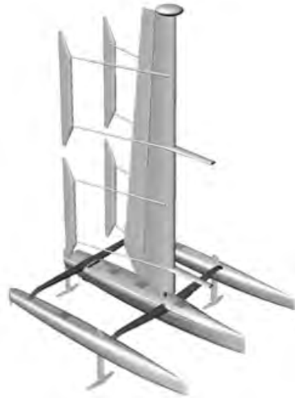
Figure 3.2: The Harbor Wing Technologies X-3 utilizes wind energy to reach speed in excess of 25kt and ranges of 500nm. Its design is well suited for offshore applications with high persistence requirements, stating a time at sea of three plus months. From [10].
