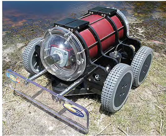
Figure 2.5: ONR’s HULLBug promises to reduce vessel’s maintenance cost by autonomously cleaning bio-fouling from the ship’s hull at regular intervals in lieu of the existing need for expensive drydocks and harsh anti-fouling coatings. From [8].
