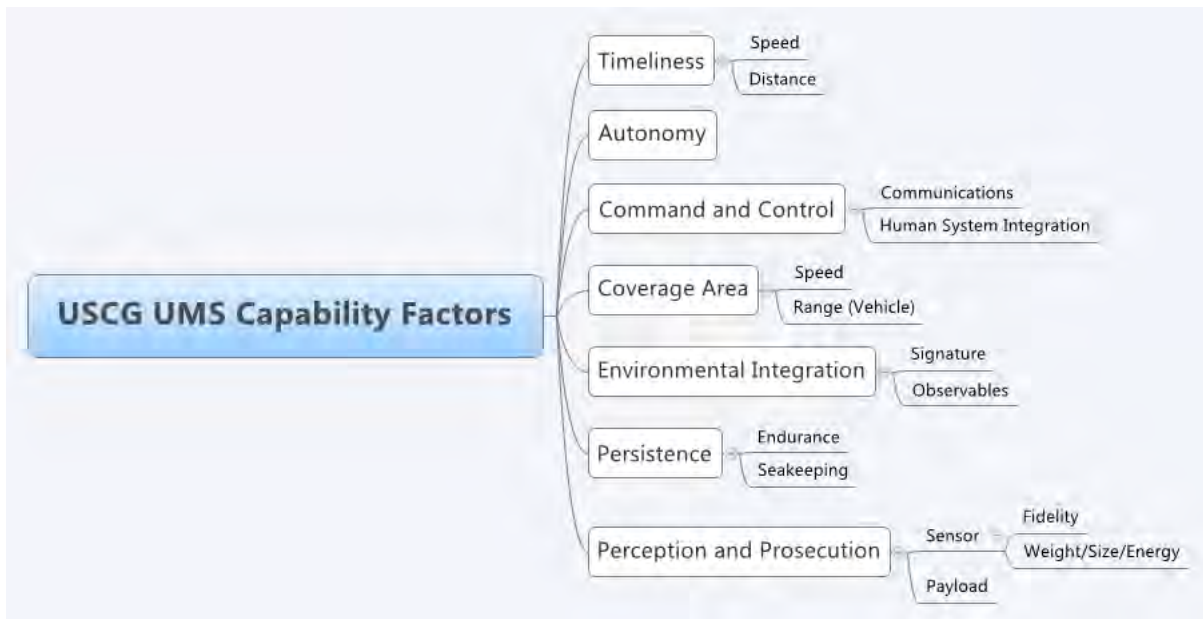
Figure 2.2: This taxonomy of capability factors describes the characteristics of mission packages and their needs. The capability factors with the most commonality across mission packages provide input for UMS alternative’s domain and characteristics.
