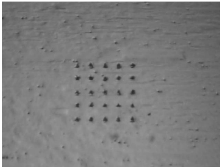
Figure 15. 5x5 indentation pattern for HT9A.
