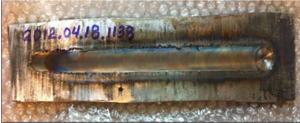
Figure 4. The friction stir welded HT9A plate, 12.7cm in length, with 8.9cm weld path.
