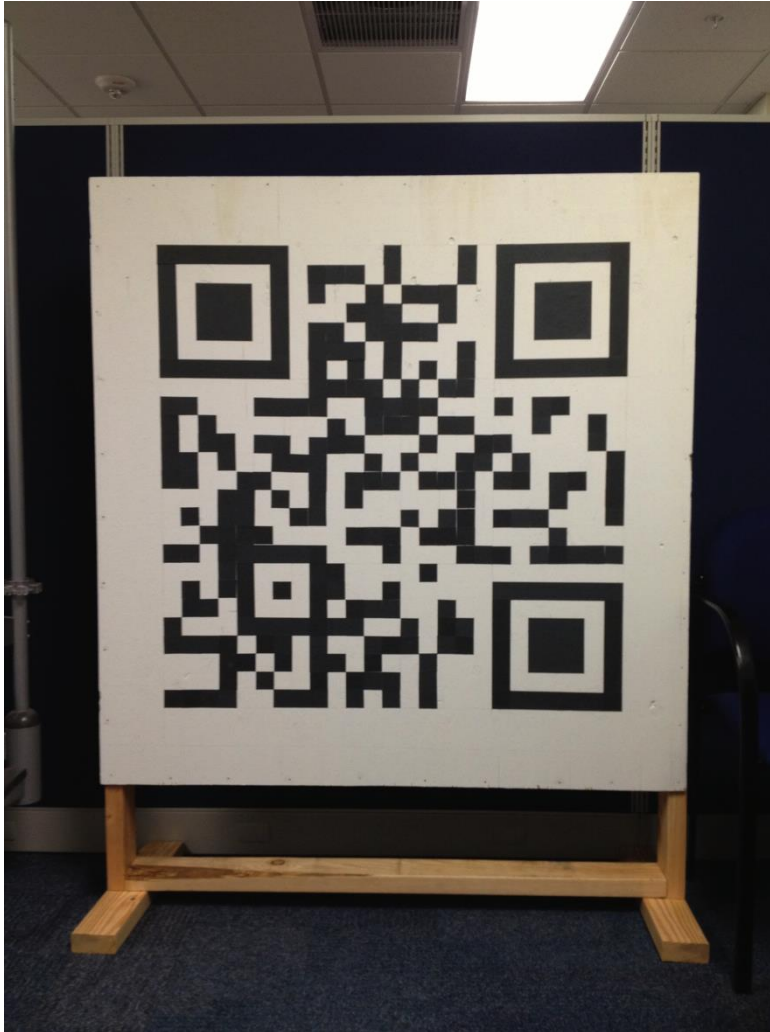
Figure 19. Field testing QR display stand constructed of basic lumber and plywood. Test QR code image: “From technical to tactical.” Version 2, ECC L(7%), 25 x 25 QR bits, 37.5 inches x 37.5 inches.
