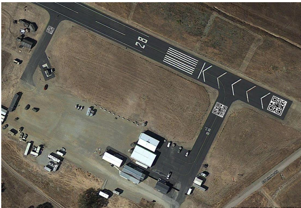
Figure 33. Artist's depiction of potential QR code locations at McMillan airfield using commercial open-source overhead imagery (After http://maps.google.com ).
