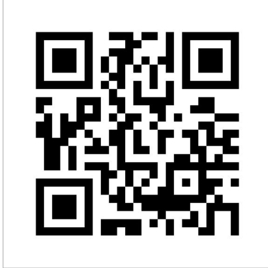
Figure 18. Test QR code image: “From technical to tactical.” Version 2, ECC L (7%), 25 x 25 QR bits. Note the necessary standards-compliant inclusion of the quiet zone 4 QR bits wide.
