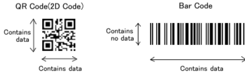
Figure 7. General characteristics of a 2D QR code compared to a 1D traditional barcode (From Sutheebanjard & Premchaiswad, 2010).
