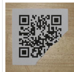
Damaged but still decodable QR code
