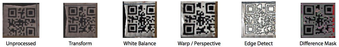
Figure 45. Process steps showing the iterative improvements of a raw captured image resulting in a readable QR code.
