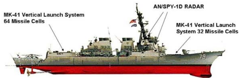
Figure 2. USS OSCAR AUSTIN (DDG 79). Note: This is the First Flight IIA, commissioned August 2000 (Source: From Global Security.org, 2006)
