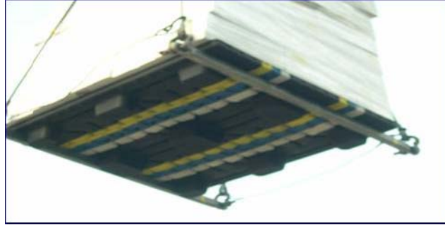
Figure 14. Navy/GSA Non-wood Pallet with Load Being Hoisted aboard Ship (Naval Inventory Control Point, 2006)
