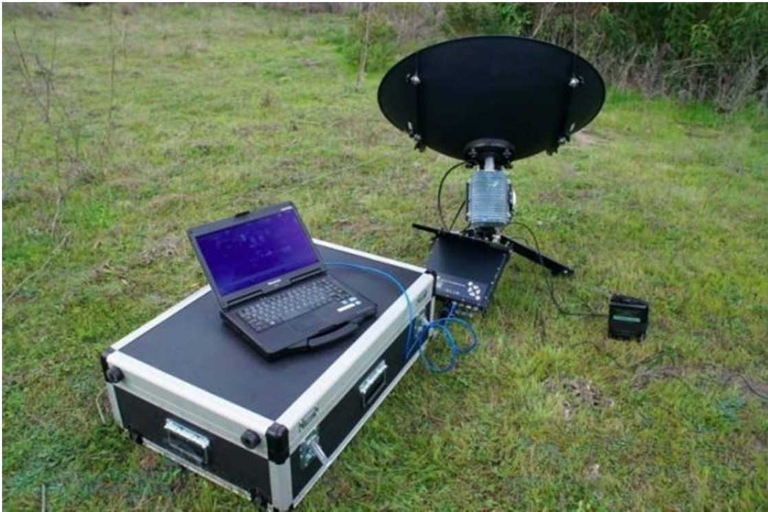
Figure 2. ViaSat Surfbeam 2 Pro Portable VSAT (From Honig, 2012)
