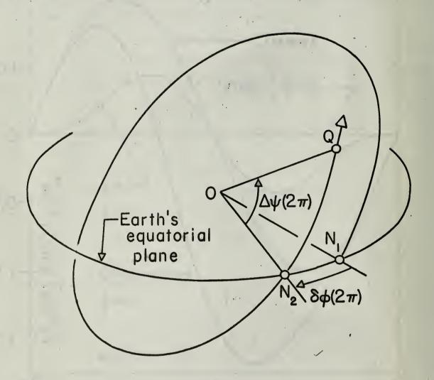
FIG. 5. Regression  $\delta \phi(2\pi)$  of the ascending node in the equatorial plane and precession  $\Delta \psi(2\pi)$  of the perturbed orbit.
