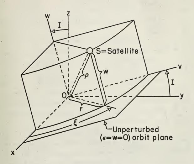
FIG. 1. Cylindrical coordinates based on the Oxv plane of the unperturbed orbit.
