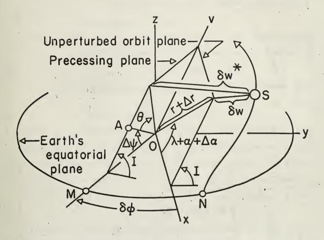
FIG. 3. Satellite variations δw out of the unperturbed orbit plane and δw\* out of the precessing perturbed orbit plane.
