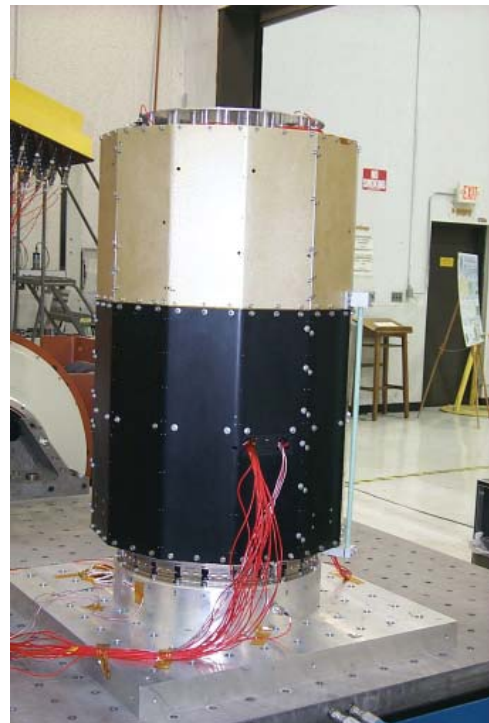
Figure 6. NPSAT1 EDU Vibration Test (Photo courtesy Naval Research Laboratory).
