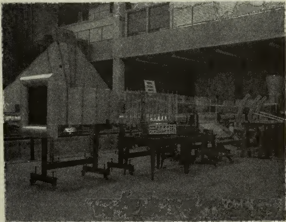
Figure 5. Overall View of Variable Pressure Gradient Subsonic Wind Tunnel
