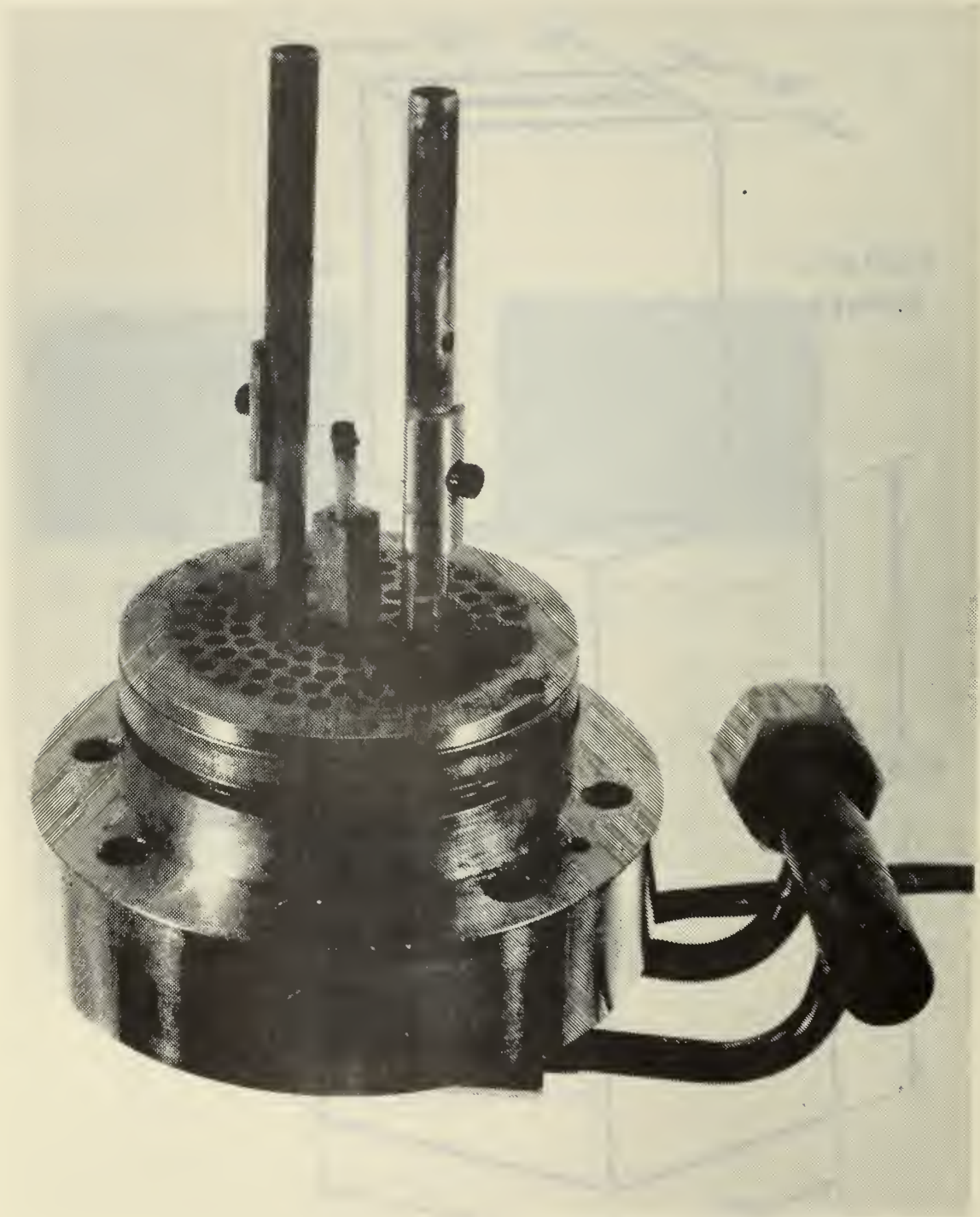
Figure 5 Combustion Bomb End Cap with Sandwich Burner Mounted
