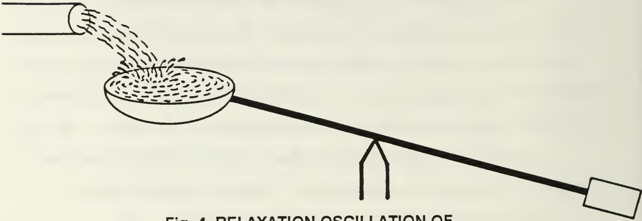
Fig. 4 RELAXATION OSCILLATION OF A SIMPLE WATER CLOCK.
