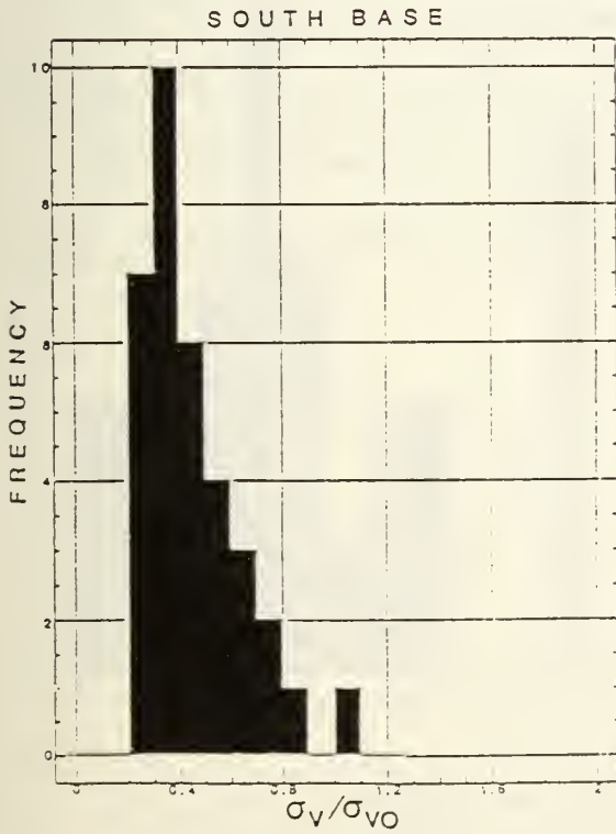
Fig. 19 The ratio of the measured boundary layer average cross wind turbulence to that assumed for flat terrain (.6 w*).
