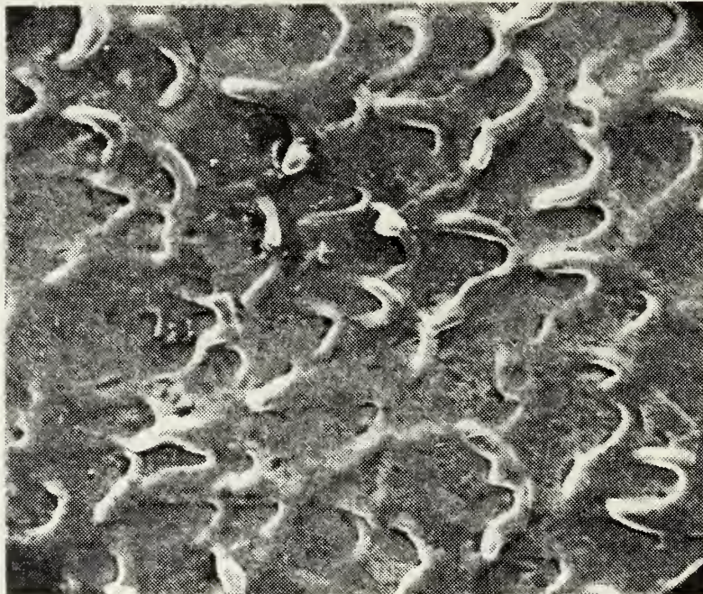
Figure 3. Flow pattern 3mm from laser impact point which is to the right of figure. Magnification 700X.
