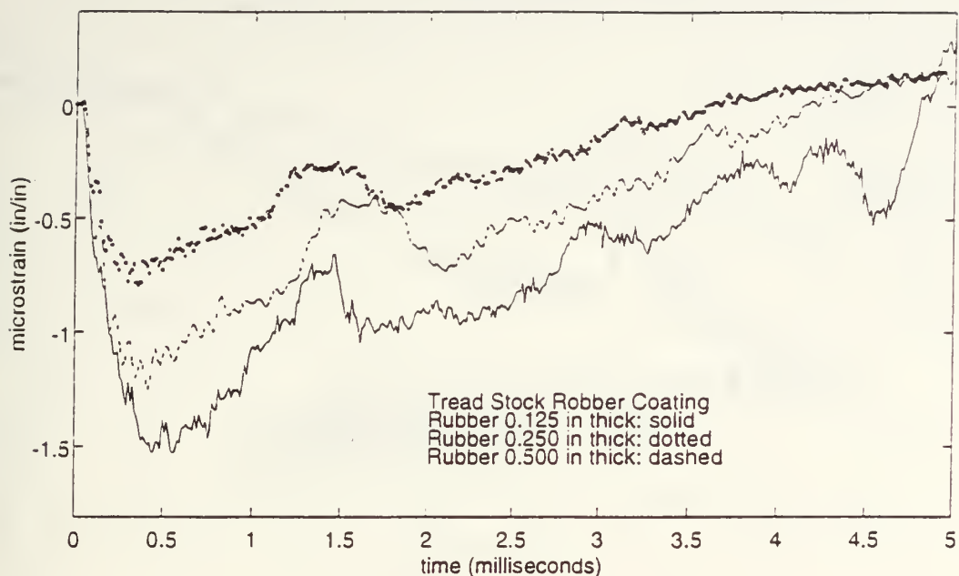
Figure 57. Hoop strain at position B for rubber-coated aluminum cylinders of varying coating thicknesses
