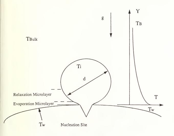
Figure 2. Model of Bubble During Growth
