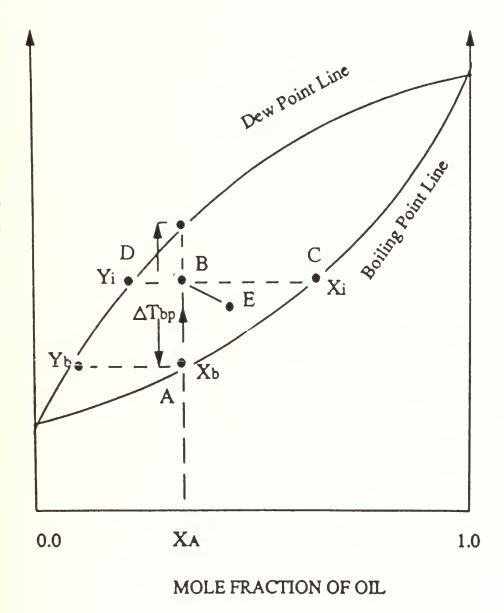
Figure 1. Vapor-Liquid Equilibrium Diagram
