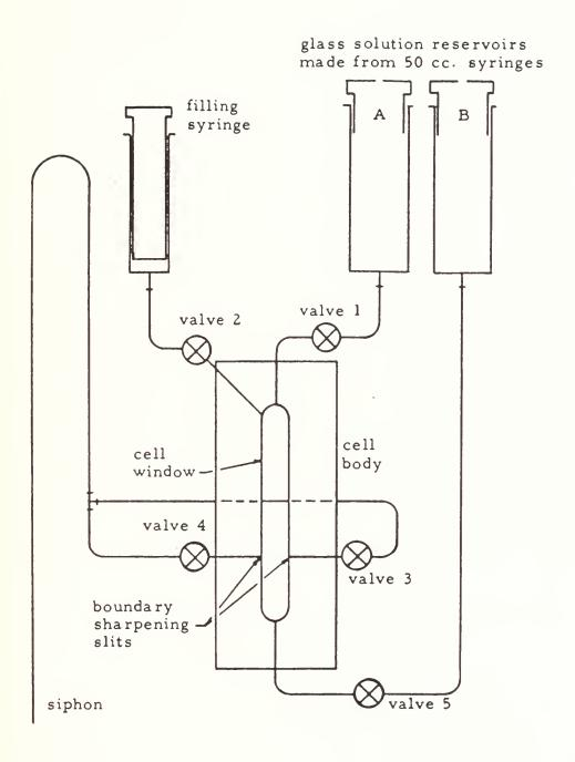
Figure 3. Diagram of Diffusion Cell (From Reference [16])
