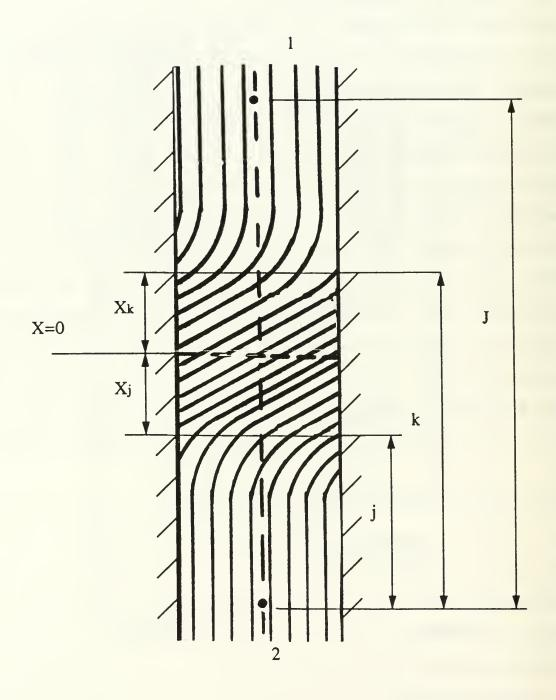
Figure 4. Schematic of Typical Interferogram at Time t (From Reference [16])
