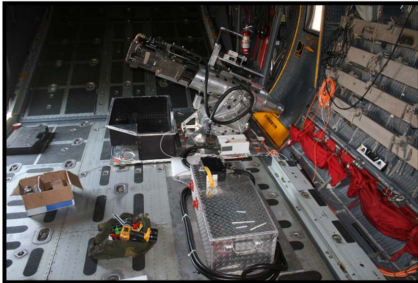
Figure 22. Picture of the Gunship in a Box roll-on/roll-off 30mm gun pointing out rear troop compartment door.
