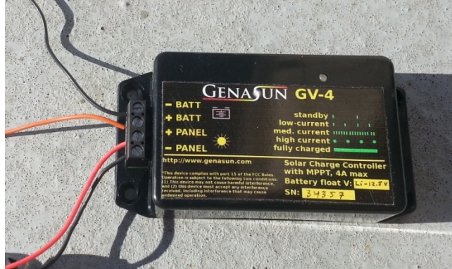
Figure 36. The Genasun-4 MPPT with DC-DC buck converter and charge controller.
