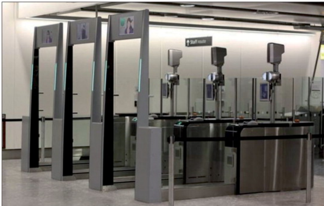
Figure 26. Photo of e-Passport gates at Terminal 4 in London's Heathrow Airport (Facial, Fingerprint and Iris), from Accenture, 2012
