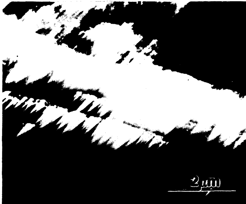
Figure 19. TEM Images of As-quenched HSLA-100 Steel Retained Austenite: \bar{B} close to \langle 133 \rangle , \bar{g} = 110 type; (Top) Bright field, (Bottom) Dark field.
