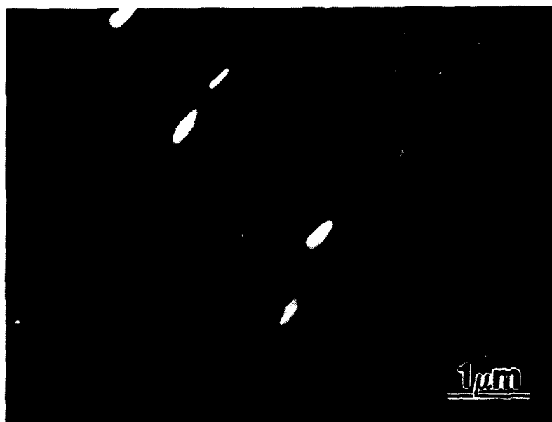
Figure 44. TEM Image of Lath Boundary Copper Precipitates in 677°C Aged HSLA-100 Steel: (Top) Bright field, (Bottom) Dark field. Micrographs taken well away from a low index pole to illuminate copper precipitates. Drift due to long exposure time required.
