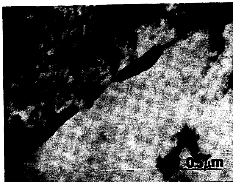
Figure 41. TEM Images of 677°C Aged HSLA-100 Steel Interlath and Intralath Carbides: Carbides too small to generate SADP.
