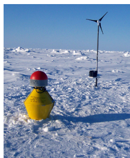
NPS-designed arctic autonomous ocean-turbulence buoy beams data to NPS, thence to internet
