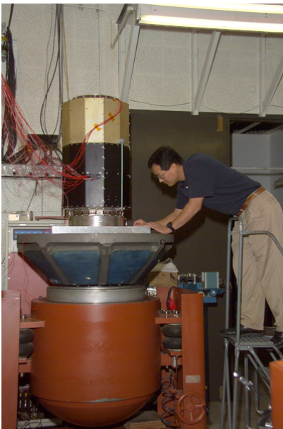
NPSAT1 demonstration satellite engineering-development unit under vibration testing, Naval Research Lab, 9/2005.
