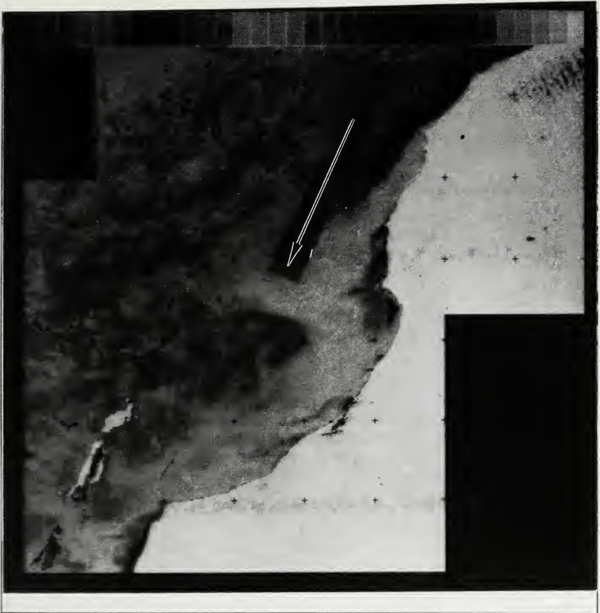
Figure 24. AVHRR image of a cold filament off NW Africa on 2 July 1985: The black crosses indicate 1° squares with north toward the top. Shades of grey are indicative of sea surface temperature, a scale in °C is provided across the top (From Nykjaer et al.,1986). The arrow indicates location of coldest water in the filament.
