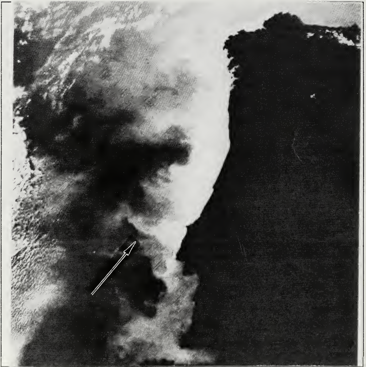
Figure 27. AVHRR image of a cold filaments off the coast of Portugal on 21 AUG 1979.: The arrow indicates the best defined filament. This cold filament extended approximately 150 km offshore. The coldest water is white and the darker shades are warm. The Straits of Gibraltar are at the top (From Fiuza, 1985).
