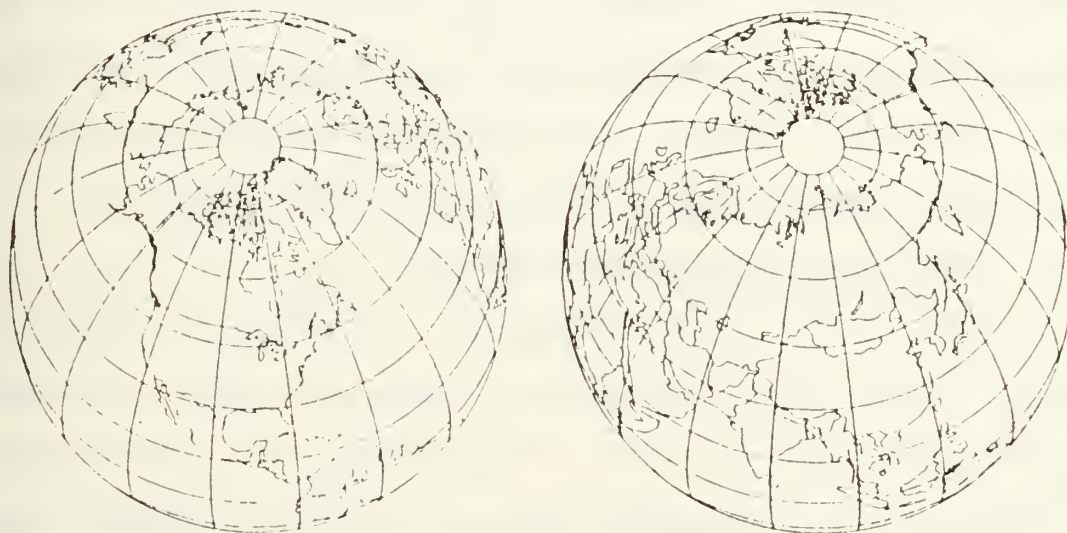
Figure 4-4. Coverage Area As Observed From A Satellite In A Molniya Orbit
