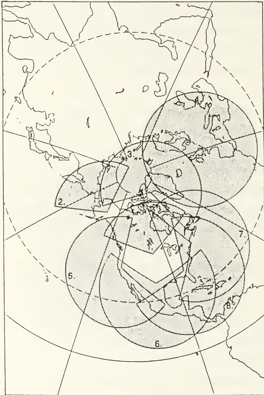
■ 1. PARCS; 2. BMEWS, Clear, Alaska; 3. BMEWS, Thule, Greenland; 4. BMEWS, Fylingdales, England; 5. PAVE PAWS, Beale AFB, California; 6. PAVE PAWS, Goodfellow AFB, Texas; 7. PAVE PAWS, Cape Cod AFS, Massachusetts; 8. PAVE PAWS Robins AFB, Georgia. Figure shows 1,000-km altitude detection contours.
