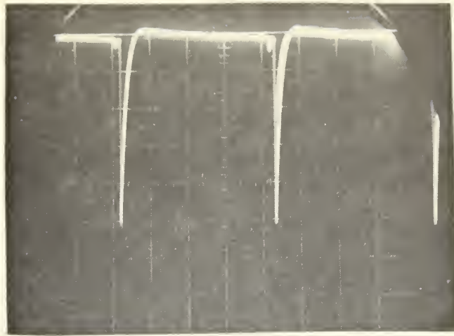
(a) Detected response of experimental MFD DF system to signal #4 (Table VII). Transmitter at 21.74 MHz.
