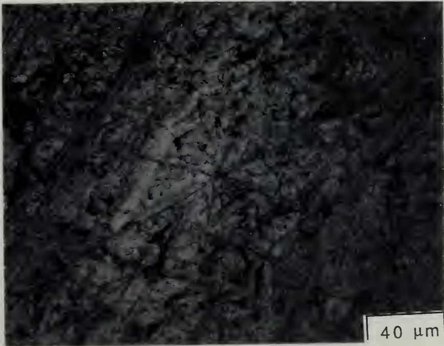
Figure G-7 Sharp features in 316 stainless steel exposed to deionized water for 96 hours at 300°C, 241.5 atm (500 x, light microscope)
