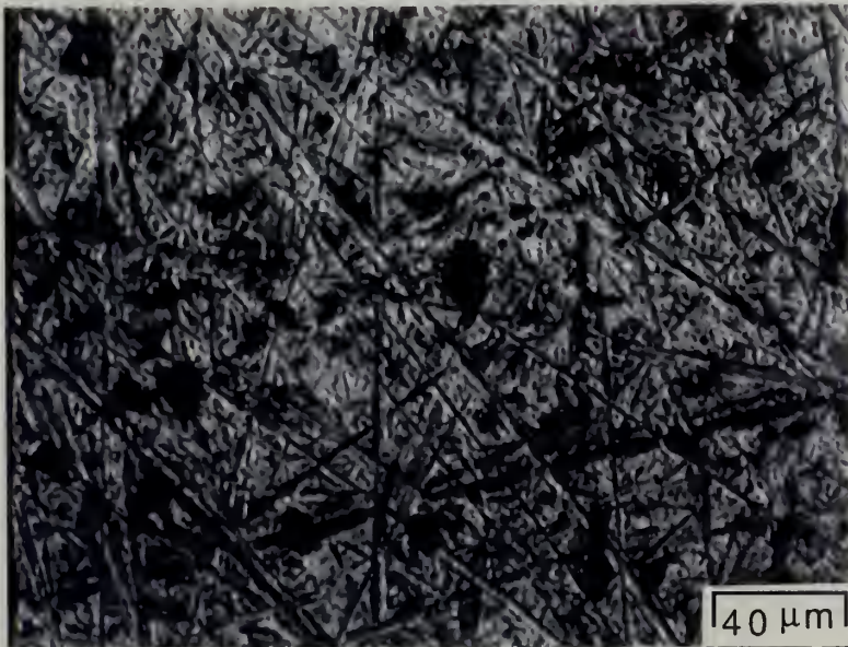
Figure G-4 Laser confocal microscope view of Inconel 625 exposed to deionized water for 96 hours at 300°C, 241.5 atm (400 x)
