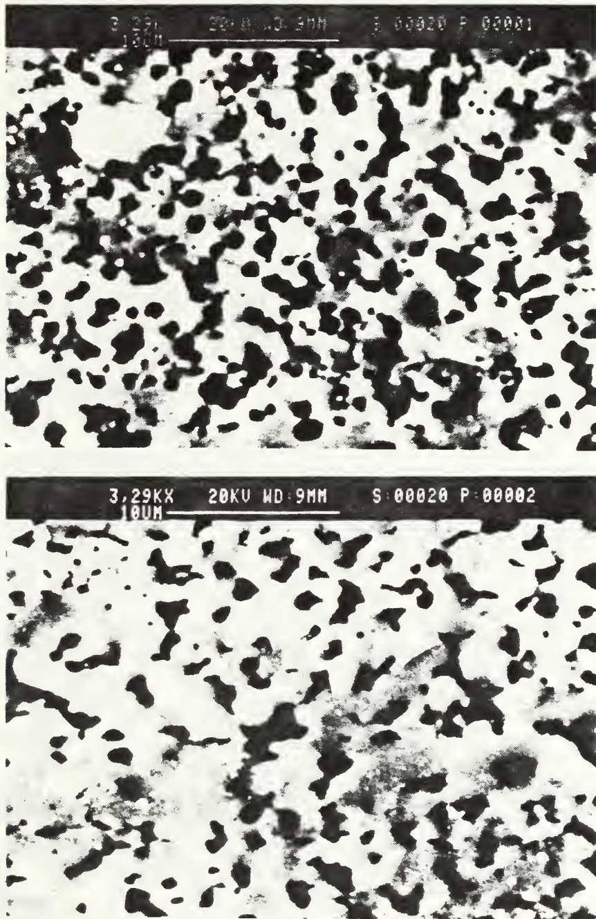
Figure 18. Electron Micrograph of TMP8 at \dot{\epsilon} = 6.11 \times 10^{-2} \text{sec}^{-1} : Interrupted tensile test specimen at \epsilon = 0.379 . Grip section shown (above), gage section shown (below).
