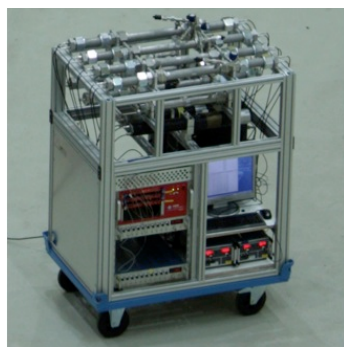
Figure 4. Array of seven ^4\text{He} detector modules.
