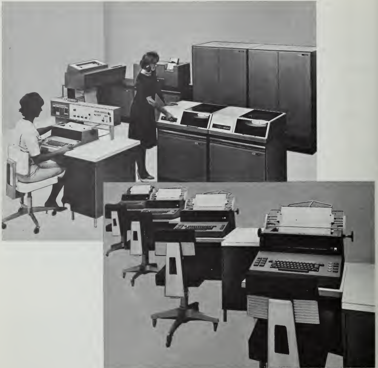
Figure 2. IBM 1440 as Control Center for IBM 1050 System Terminals
