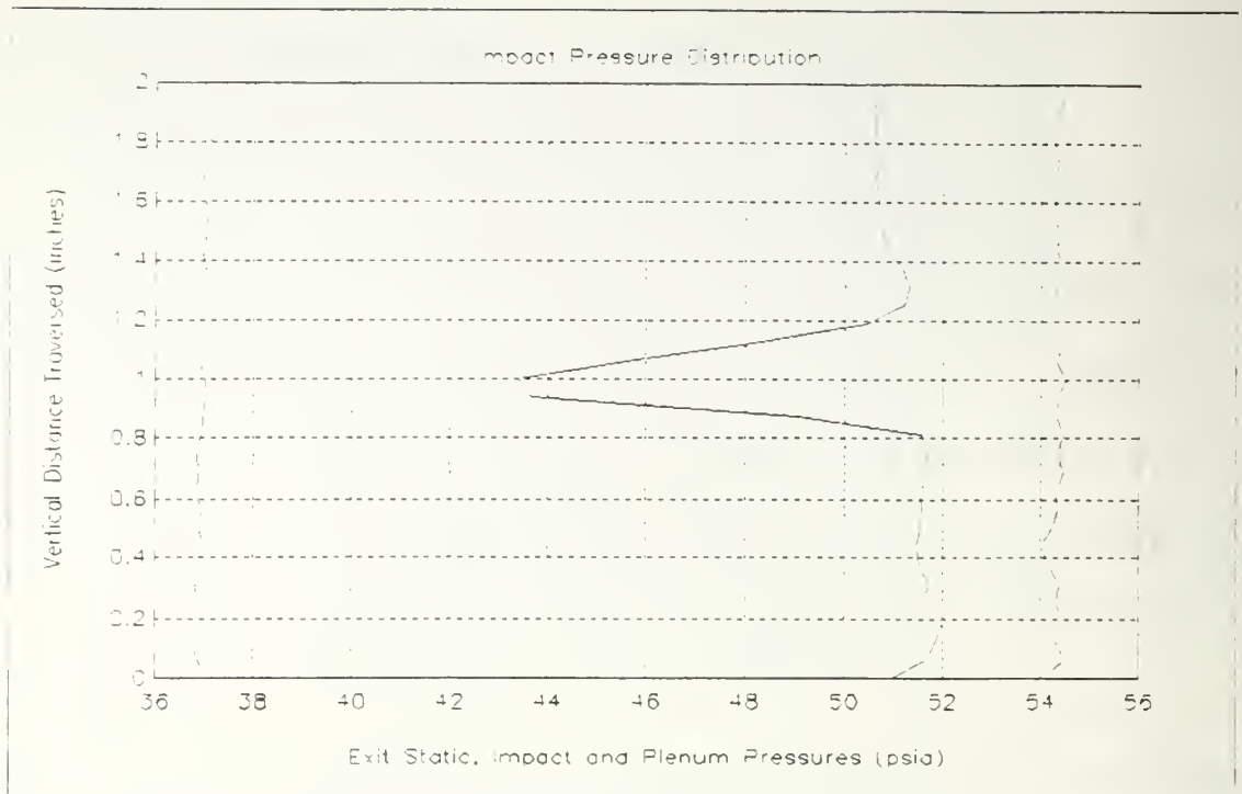
Figure 22. Loss Distribution at Design Incidence (1.15 degrees)
