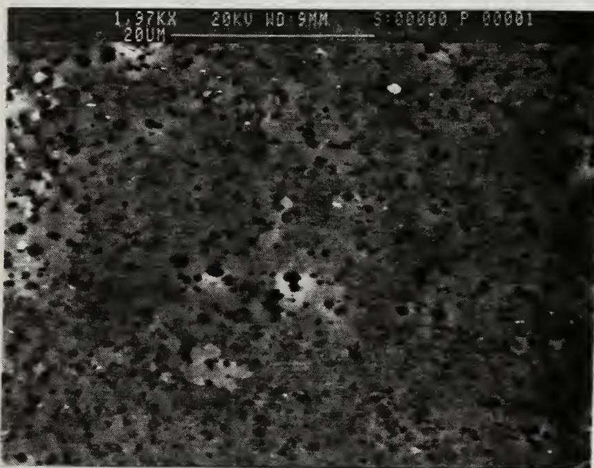
Figure 13. Backscattered SEM micrograph showing Al-10Mg-0.1Zr alloy following pass 12 of TMP 7: a) in the as-rolled condition; b) following 30 minutes of annealing at 300°C.
