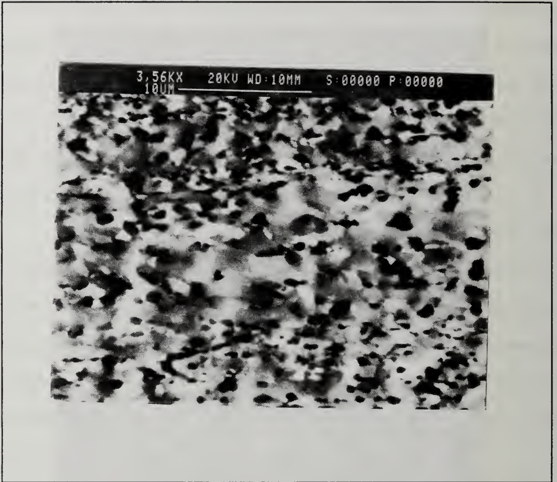
Figure 11. Backscattered SEM micrograph showing Al-10Mg-0.1Zr alloy following pass 8 of TMP 6: c) in the annealed condition at a higher magnification.
