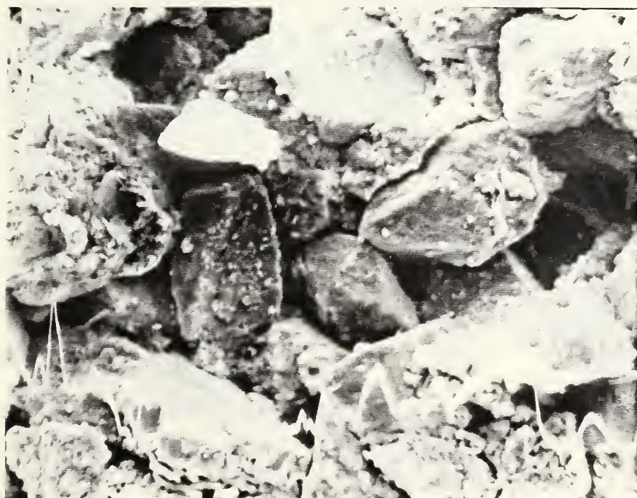
Figure A-12: Frio Sandstone, 9189.5 ft, x100, x250
