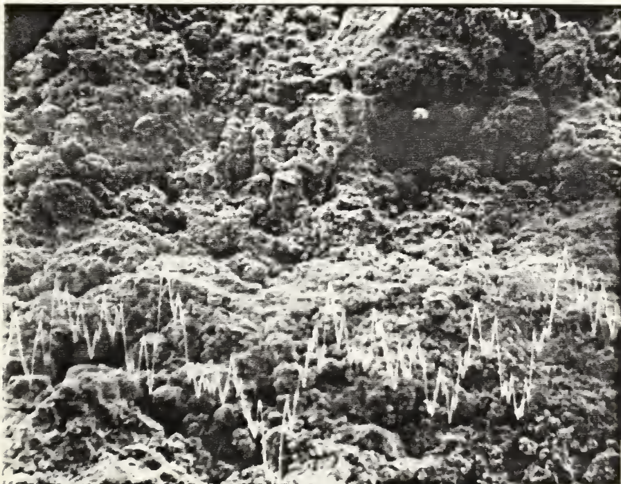
Figure A-23: San Andres Dolomite, 3464ft, x27, x54
