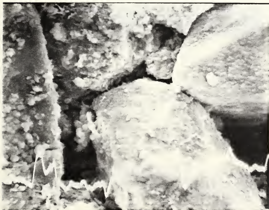
Figure A-13: Frio Sandstone, 9189.5 ft, x510, x750
