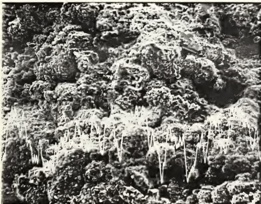
Figure A-17: San Andres Dolomite, 3350ft, x31, x54
