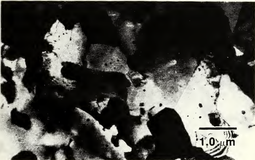
Figure 4.21. Bright field TEM micrographs of alloy 2090 from the gage section of a tensile sample tested at 300°C and 6.67 \times 10^{-4} \text{ S}^{-1} strain rate.
