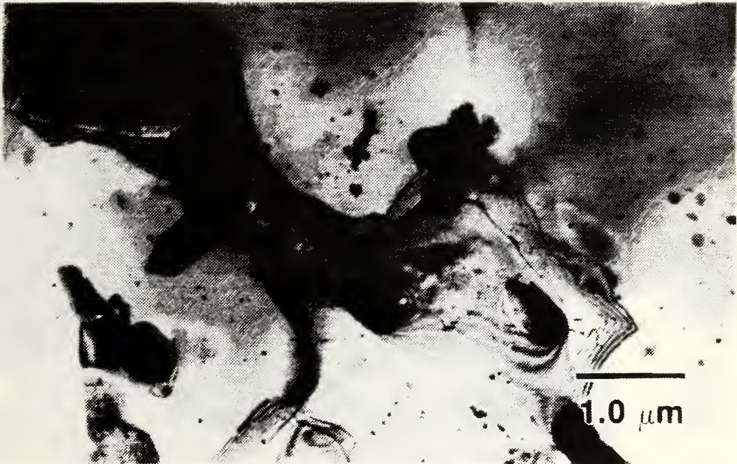
Figure 4.23. Bright field TEM micrographs, of alloy 2090 from the gage section of a tensile sample tested at 300°C and 6.67 \times 10^{-4} \text{ S}^{-1} strain rate processed by TMP 6.
