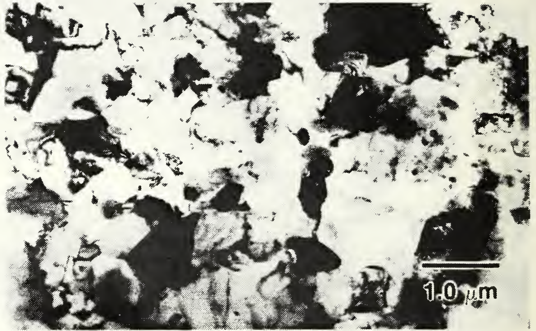
Figure 4.10. Bright field TEM micrograph, of alloy 2090 in the as-rolled condition processed by TMP 6.
