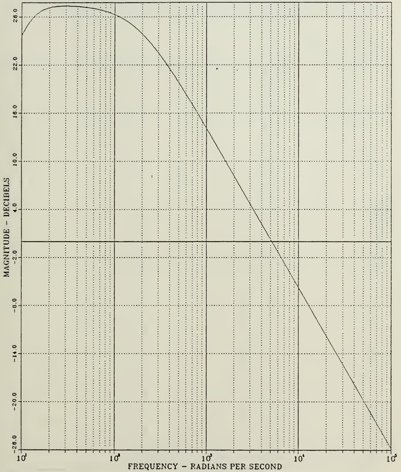
Figure 2.12 Pitch Angular Rate; Uncoupled Pitch Channel; Continuous Open Loop System; Gain vs Frequency.
