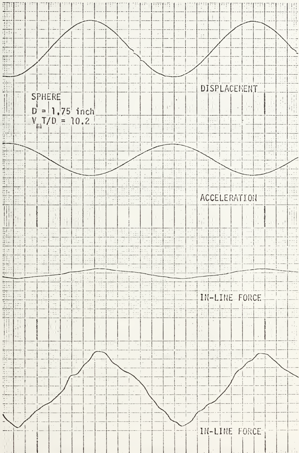
Figure 9. Force, displacement traces.
