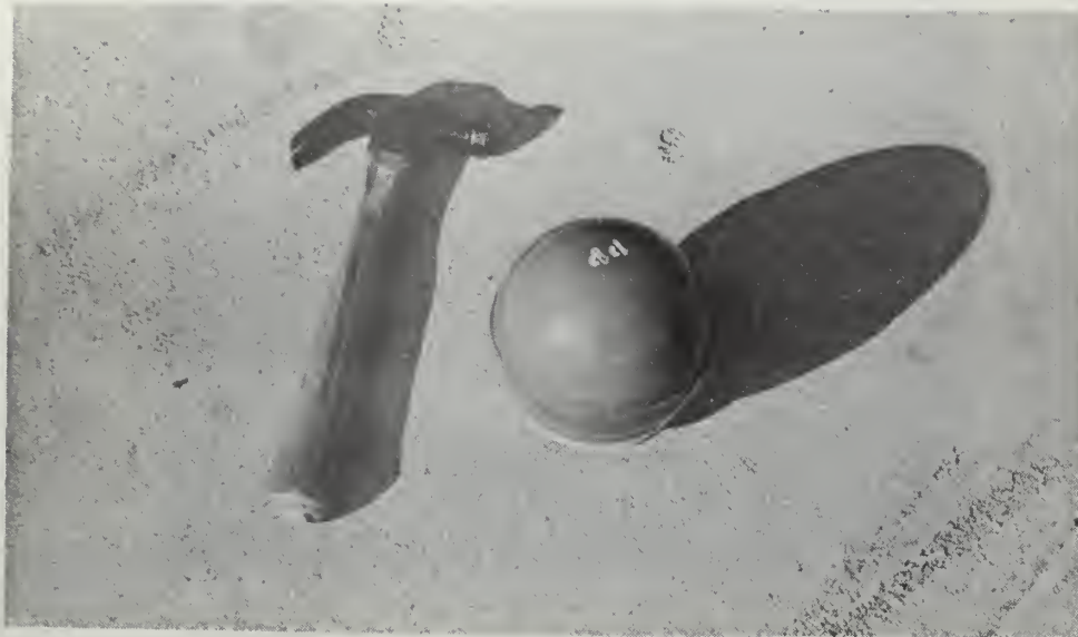
Figure 6. ECCO Radar Reflector
