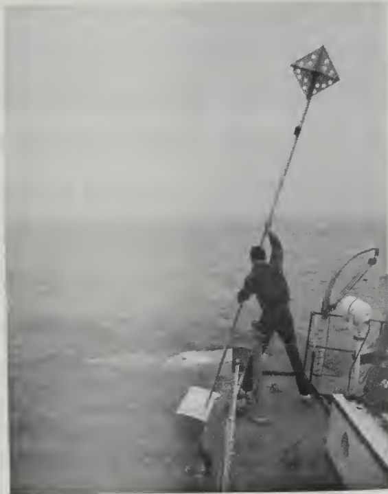
Figure 9. Launching Surface Float Assembly
