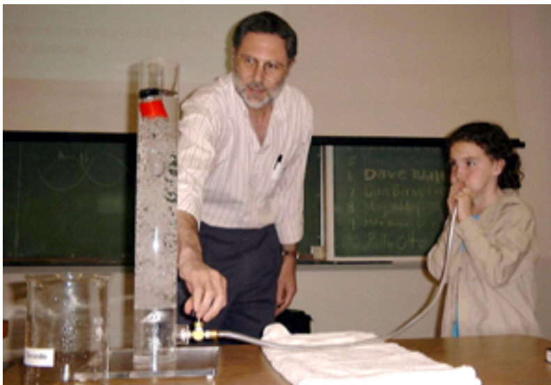
Figure 2. Demonstration apparatus for sinking a body with bubbles, being operated at a section meeting of the American Association of Physics Teachers [6]. The volunteer is the daughter of a physics professor, and the author is controlling the valve.
