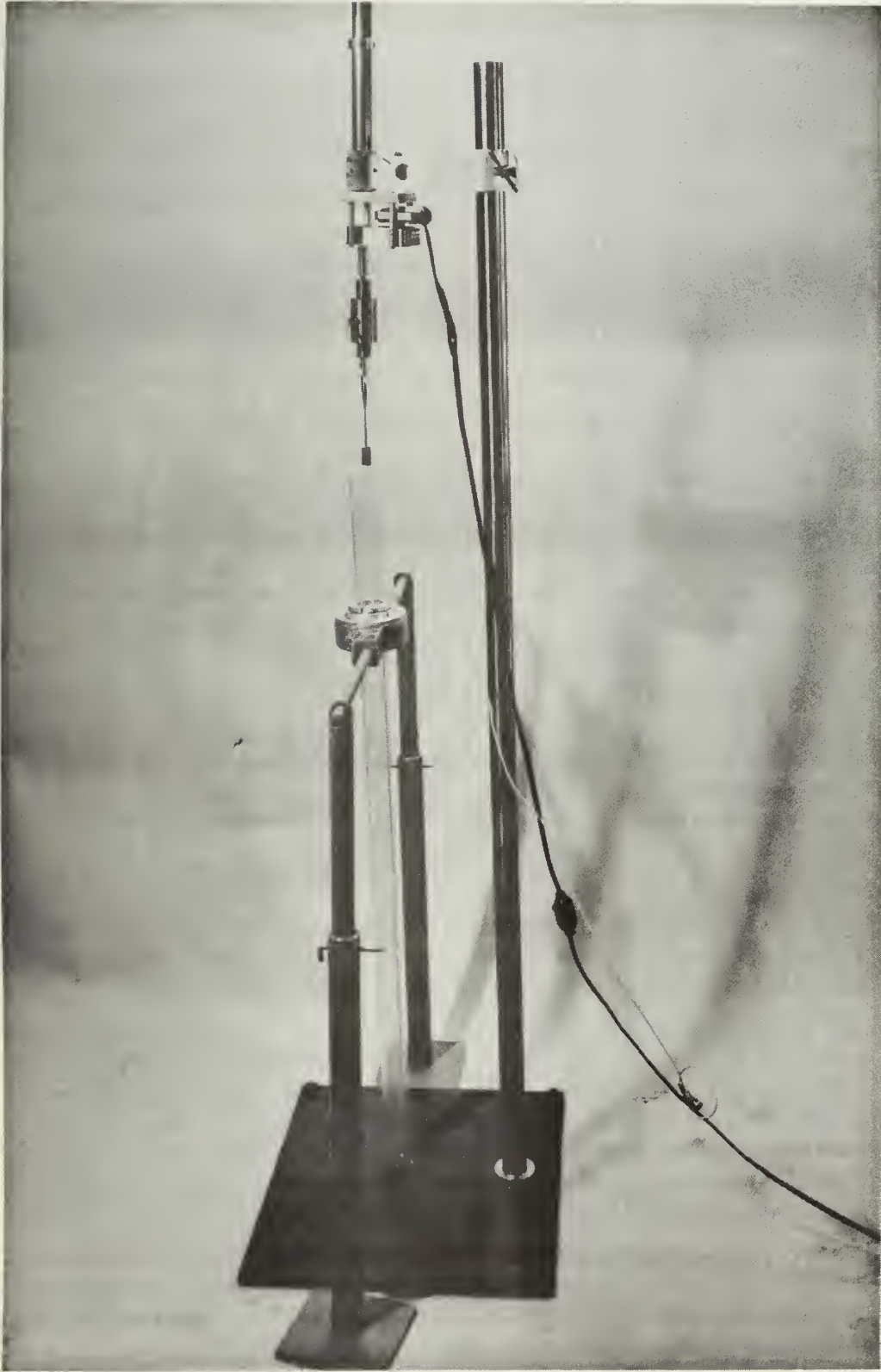
Figure 4. The PGS Vane-Shear Apparatus, shown in the Shipboard Configuration
