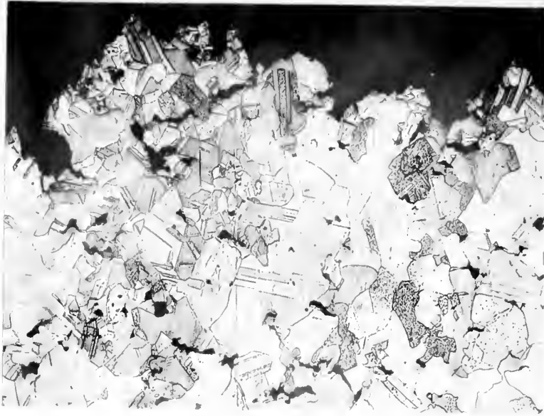
Fig. 37 - Photomicrograph of the fracture area of specimen G-1B; 500° C., 4,000 psi, 0.28 in./in. rupture strain, and fracture time of 21.2 hours. (100 X)
