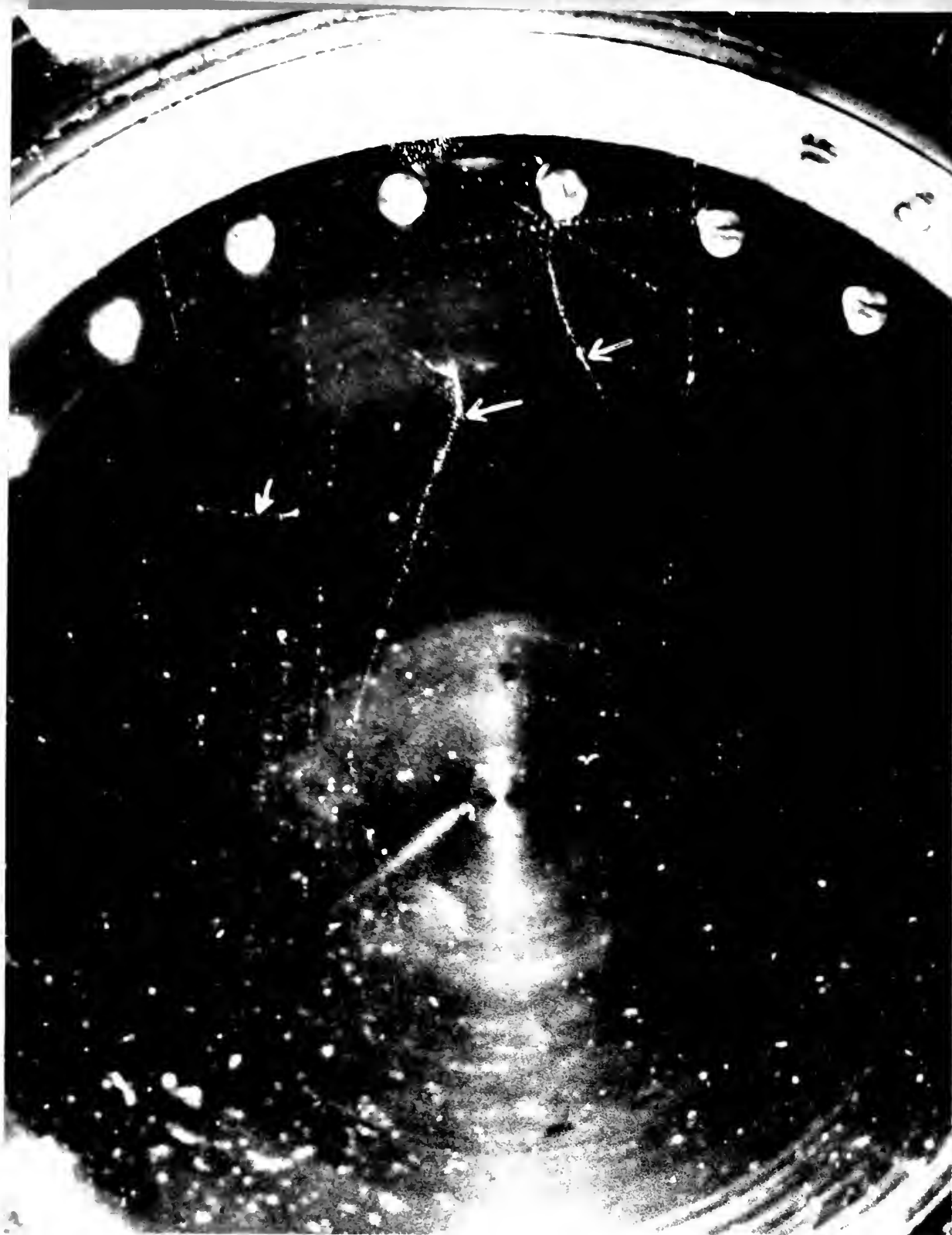
Figure 21 PROTON TRACKS IN NITROGEN
