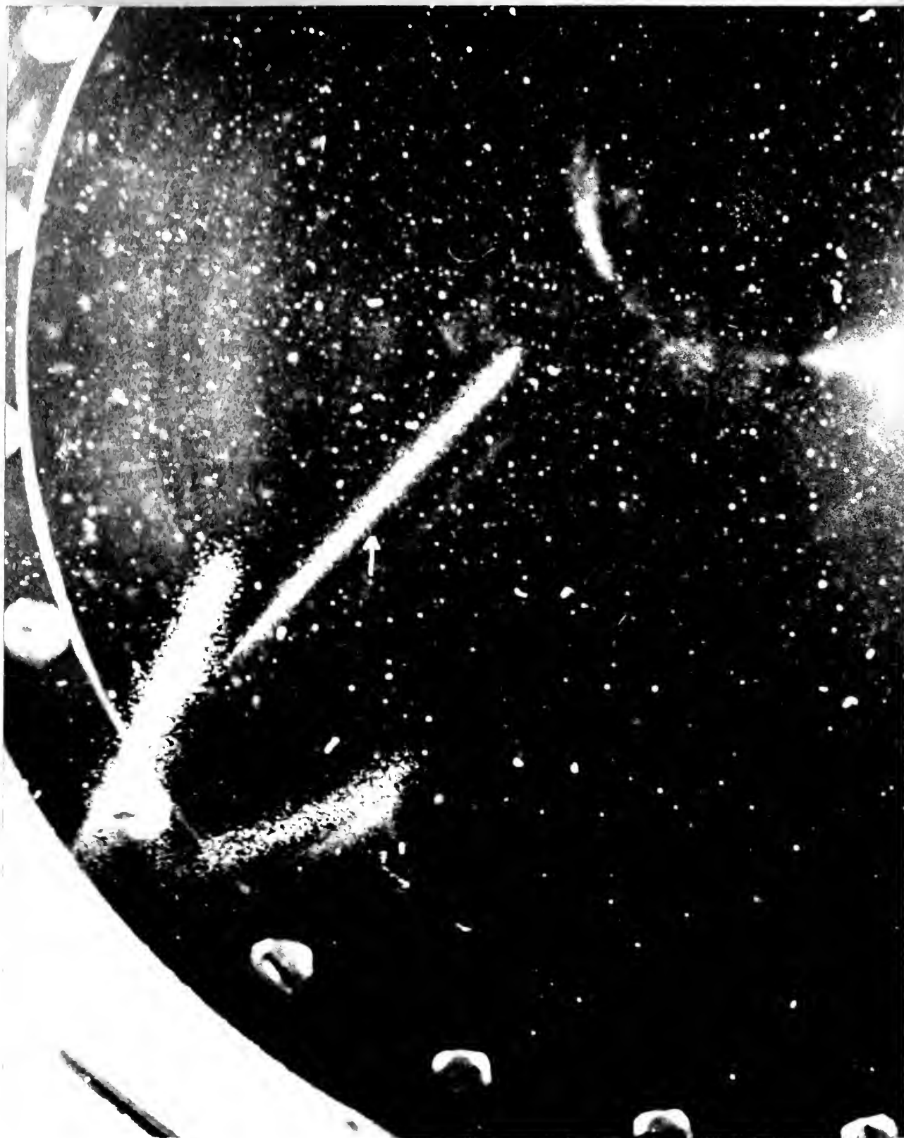
Figure 17 ALPHA TRACKS IN HELIUM FROM \text{Po}^{210} SOURCE
