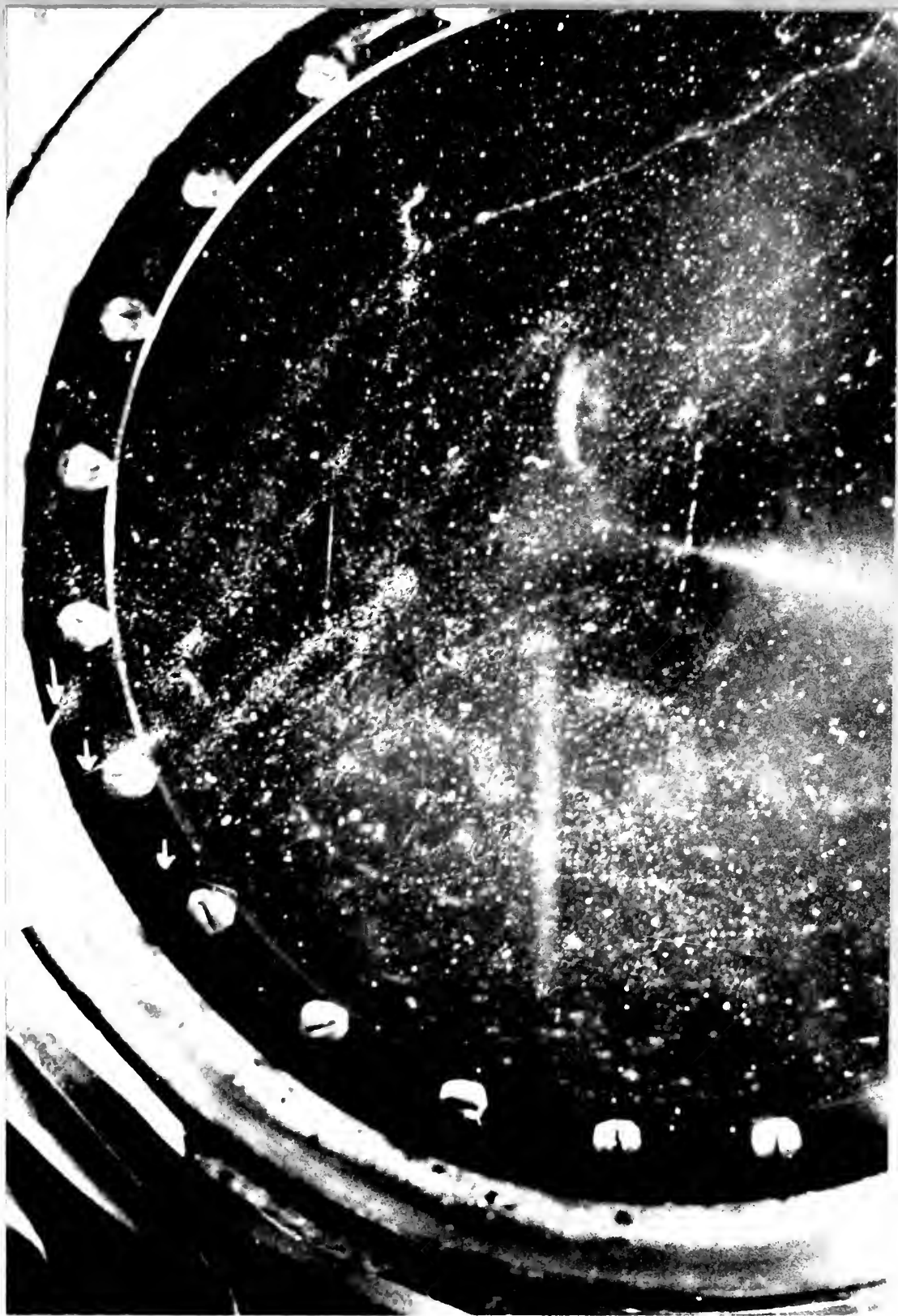
Figure 18 ALPHA (From \text{Po}^{210} ) AND BETA (From \text{Bi}^{210} ) TRACKS IN NITROGEN
